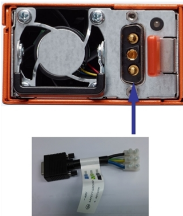
Figure 4 Connecting DC Power Supply Module
