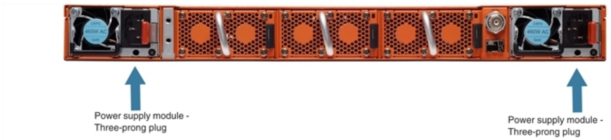
Figure 2 Connecting AC Power (GigaVUE-HC1)
